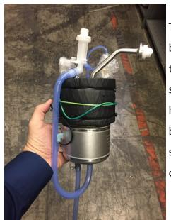
The new style tank will be different from the old tank. It may be necessary to drill out the screw holes on the mounting bracket slightly as your screws may be a slightly different size.
