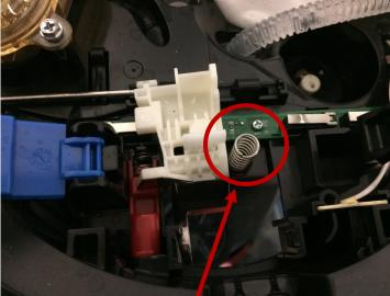
Pull the old handle up and out and insert the new one making sure to line up the spring underneath with the insert on the bottom of the handle. Slide the pin back into place.
