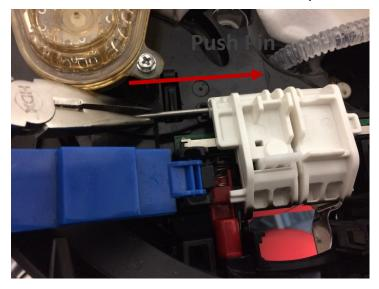
Put the clear outlet with the hot tube back into place. Turn the SmartFlo back into position and install into place. Turn the blue clips to lock it down and snap the latch into place. Close the cabinet top.
