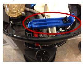
Locate and turn the blue locking clips so that the SmartFlo can be pulled up and rotated to the right so that it is out of the way. Locate and remove the transparent outlet between the faucet handles by gently pinching the tabs and pulling up and out of the way to the left.
