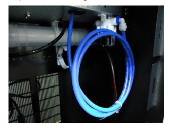
CAUTION: All connections must have the supplied locking clips installed.
