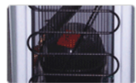
Hermetically sealed reciprocating Compressor
