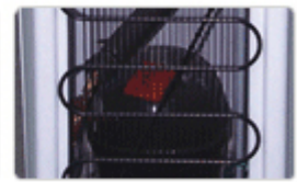
Hermetically sealed reciprocating Compressor
